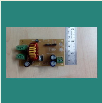
Solar Charge Controller with LED Driver
